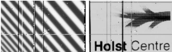
Examples of X-ray image (left) and optical image (right) obtained with Holst Centre's X-ray detector on plastic substrate.
