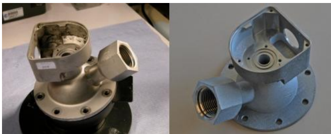
Original and 3D-printed 'woov' valve. Credit: ESA
