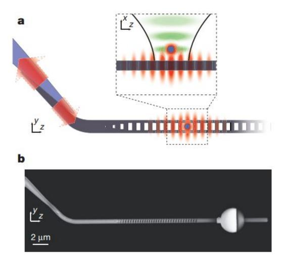
Strong coupling of a trapped atom to a photonic crystal cavity. a, A single 87Rb atom (blue circle) is trapped in the evanescent field (red) of a photonic crystal (grey). The photonic crystal is attached to a tapered optical fibre (blue), which provides mechanical support and an optical interface to the cavity. The tapered
