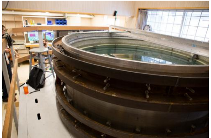
Deep water tank in the APL for testing underwater conditions.
