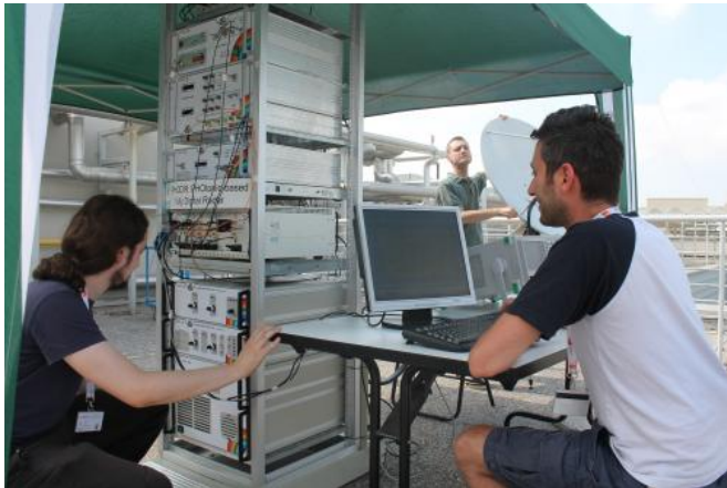
The research team while testing the photonics-based coherent radar system on the roof of the laboratory in Pisa, Italy, detecting the aerial traffic from the close airport. Credit: Antonella Bogoni
