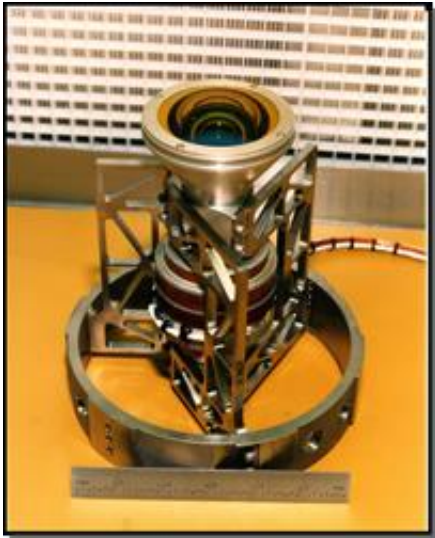
This photo shows optics in the Lightning Imaging Sensor telescope. Credit: NASA
