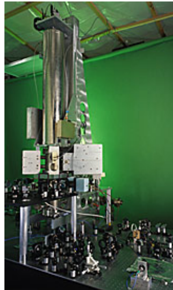
The NIST F1 clock uses a fountain-like movement of cesium atoms to determine the length of the second so accurately that--if it were to run continuously--it would neither lose nor gain one second in 80 million years. Credit: Geoffrey Wheeler Photography
