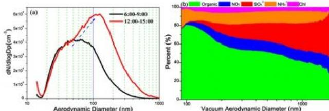
This shows a) particle number size distributions and b) fractional contributions of organics, nitrate, sulfate, ammonium, and chloride to the PM<sub>1</sub> mass during the haze episode from 06:00 to 15:00 LT, Jan. 12, 2013. Credit: Science China Press
