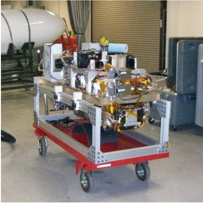
MABEL, short for "Multiple Altimeter Beam Experimental Lidar," serves as an ICESat-2 simulator. Credit: NASA/Kelly Brunt
