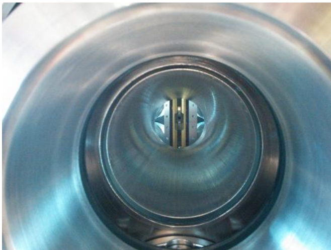
A "molecular eye" view of the vacuum chamber used for the measurement of the electron's EDM. Credit: B.R. O'Leary
