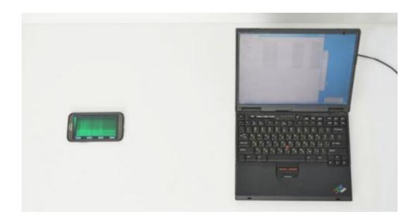
Physical setup of a key recovery attack. A mobile phone (Samsung Note II) is placed 30 cm from a target laptop. The phone's internal microphone points towards the laptop's fan vents. Full key extraction is possible in this configuration and distance. Credit: Daniel Genkin et al.
