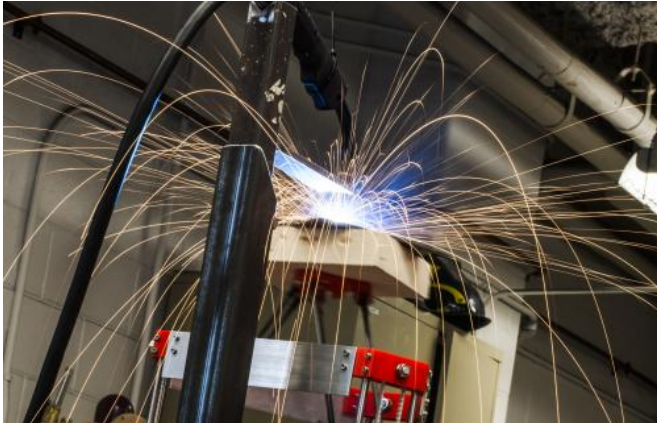
This is Michigan Tech's open-source 3-D metal printer in action. Credit: Chenlong Zhang
