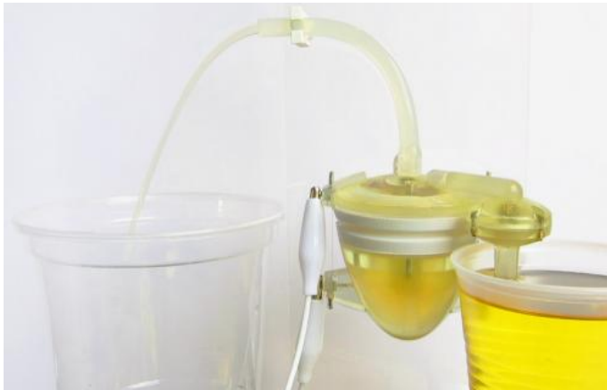
The artificial heartbeat actuator pumping urine. Credit: Walters, et al. Centre for Fine Print Research and Bristol Robotics Laboratory ©2013 IOP Publishing Ltd
