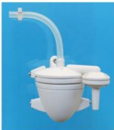
Illustration and photo of the artificial heartbeat actuator. The compressible region is made from silicone cast in 3D printed molds. Credit: Walters, et al. Centre for Fine Print Research and Bristol Robotics Laboratory ©2013 IOP Publishing Ltd
