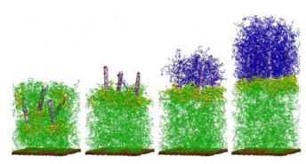
In the computer simulation, the composite is cut (far left) and the nanorods begin migration to the cut interface. In the third image, the polymerization from the rods surface and cross-linking initiates, culminating in the newly regrown gel (final image). Credit: University of Pittsburgh
