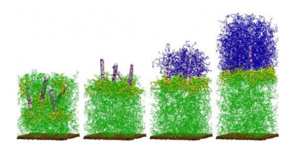
In the computer simulation, the composite is cut (far left) and the nanorods begin migration to the cut interface. In the third image, the polymerization from the rods surface and cross-linking initiates, culminating in the newly regrown gel (final image). Credit: University of Pittsburgh
