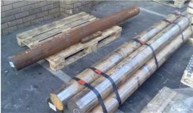
Large-scale manufacture of nanostructured steel shafts.
