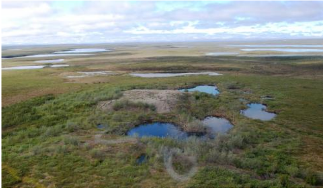
This large drilling sump exhibits ponding both on the surface and perimeter. Credit: Joshua Thienpont
