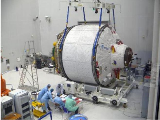
The ICC portion of the Automated Transfer Vehicle Albert Einstein, the fourth in a series of lifeline vessels bringing supplies and critical altitude boosts to the International Space Station, being weighed at Kourou space center, French Guiana
