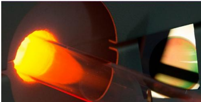
Silicon chip with porous surface next to the special furnace where it was coated with graphene to create a supercapacitor electrode. Credit: Joe Howell / Vanderbilt)
