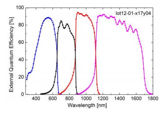
External Quantum Efficiency of the four-junction solar cell. The measurement was performed at the Fraunhofer ISE CalLab. Credit: Fraunhofer ISE
