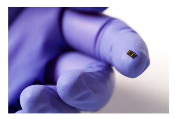
World record solar cell with 44.7% efficiency, made up of four solar subcells based on III-V compound semiconductors for use in concentrator photovoltaics. Credit: Fraunhofer ISE
