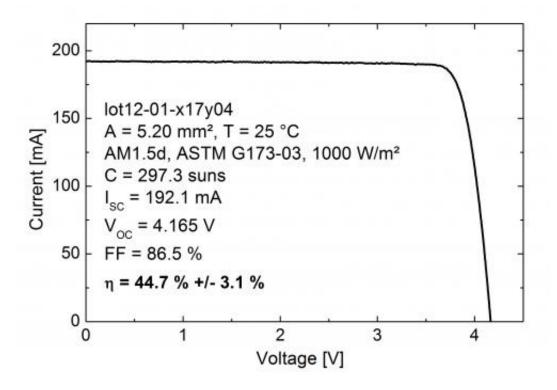
IV-characteristic for the current best four-junction solar cell under AM1.5d ASTM G173-03 spectrum at a concentration of 297 suns. The measurements were carried out at the Fraunhofer ISE CalLab. Credit: Fraunhofer ISE
