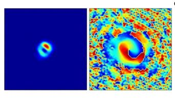
These images shows the spiral structure of the coherent OAM light emitted from a beam of electrons accelerated to nearly the speed of light and arranged into a helix by a simple laser. Left: An intensity map. Note the dark center where the light cancels itself out, resulting in a cross section resembling a doughnut. Right: A phase structure map, clearly showing the helix described by the light. Credit: Hemsing, et al.
