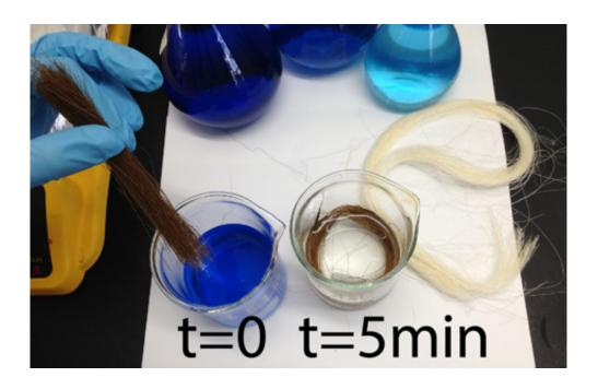
The beaker on the left contains an indigo blue dye solution prior to treatment with modified fique fibers (dark brown). The beaker on the right shows the same indigo blue solution made clear, after modified fique fibers degraded the dye in only five minutes. The image also shows raw, untreated fique fibers (off-white) on the table.
