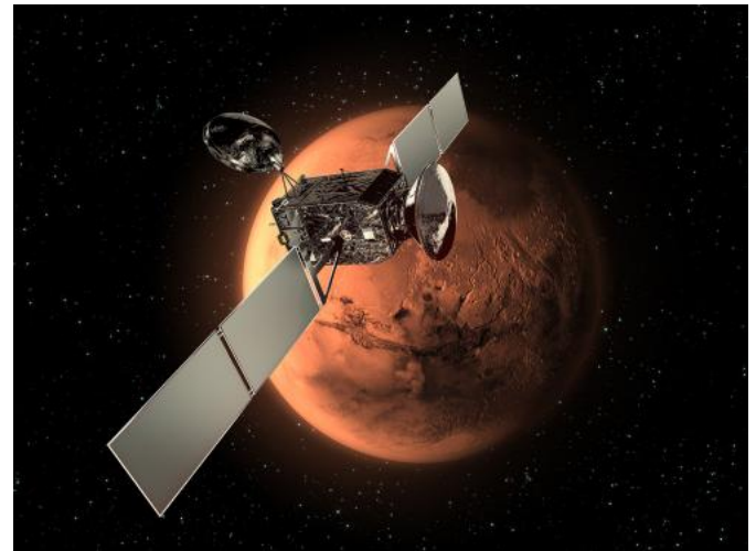
ExoMars 2016 Mission to the Red Planet. It consists of two spacecraft – the Trace Gas Orbiter (TGO) and the Entry, Descent and Landing Demonstrator Module (EDM) which will land. Credit: ESA
