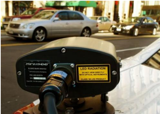
A license plate reader is mounted on the trunk of a police car in Washington, DC, on December 1, 2011.
