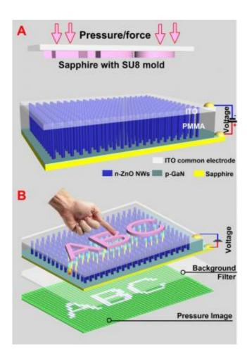
This schematic shows a device for imaging pressure distribution by the piezo-phototronic effect. The illustration shows a nanowire-LED based pressure sensor array before (a) and after (b) applying a compressive strain. A convex character pattern, such as "ABC," molded on a sapphire substrate, is used to apply the pressure pattern on the top of the indium-tin oxide (ITO) electrode. Credit: Zhong Lin Wang
