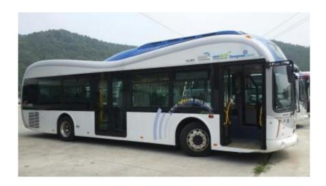
OLEV Bus is an electric vehicle that can be charged while stationary or driving. Credit: KAIST
