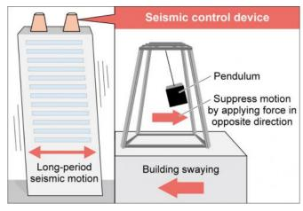
(Phys.org) —Two Japanese companies, Mitsui Fudosan and Kajima Corp, have announced plans to install quake damping pendulums atop the Shinjuku Mitsui Building in downtown Tokyo by 2015. The building, like many others in the city, was built before new quake dampening technology was developed for skyscrapers.
