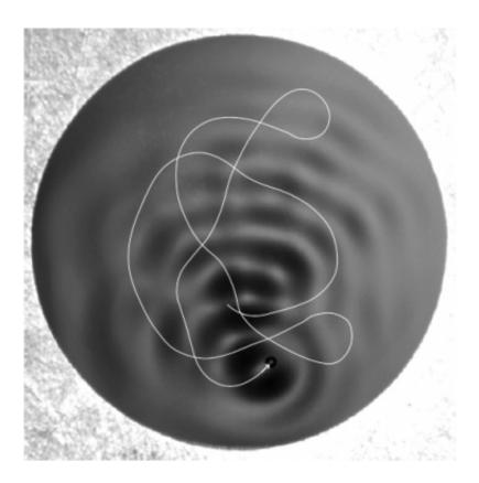
When the waves are confined to a circular corral, they reflect back on themselves, producing complex patterns (grey ripples) that steer the droplet in an apparently random trajectory (white line). But in fact, the droplet's motion follows statistical patterns determined by the wavelength of the waves. Credit: Dan Harris
