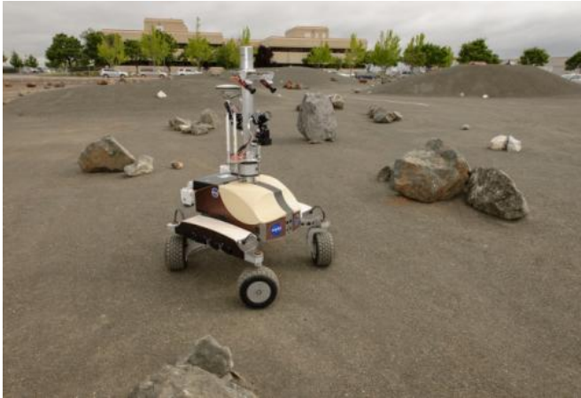
K10 Black planetary rover navigates the boulder field in the Roverscape during a Surface Telerobotics Operational Readiness Test at NASA's Ames Research Center. Credit: NASA/Dominic Hart
