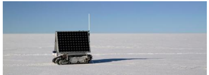
For the power test on June 2, researchers sent GROVER a list of coordinates forming a large circle outside of Summit Camp. GROVER went around the loop three times and tracked all of the waypoints. Credit: NASA Goddard/Matt Radcliff
