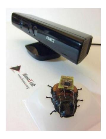
North Carolina State University researchers are using Kinect video game technology to remotely control cockroaches on autopilot, with a computer steering the cockroach through a controlled environment. Credit: Alper Bozkurt, North Carolina State University
