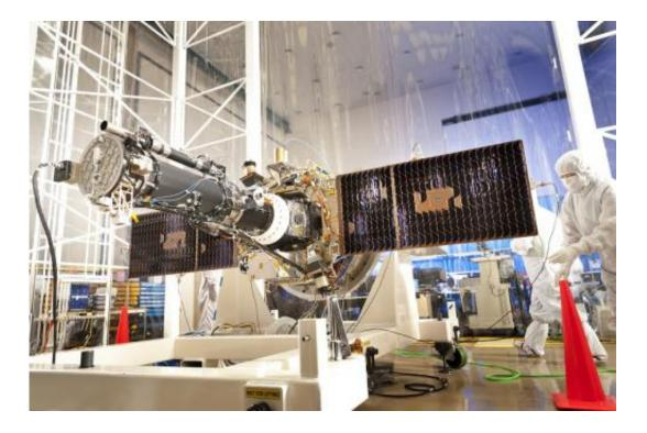
Technicians work on NASA's Interface Region Imaging Spectrograph (IRIS) in a "clean room", a specially designed facility intended to minimize contaminants on spacecraft before launch. Credit: Lockheed Martin
