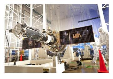
Technicians work on NASA's Interface Region Imaging Spectrograph (IRIS) in a "clean room", a specially designed facility intended to minimize contaminants on spacecraft before launch. Credit: Lockheed Martin
