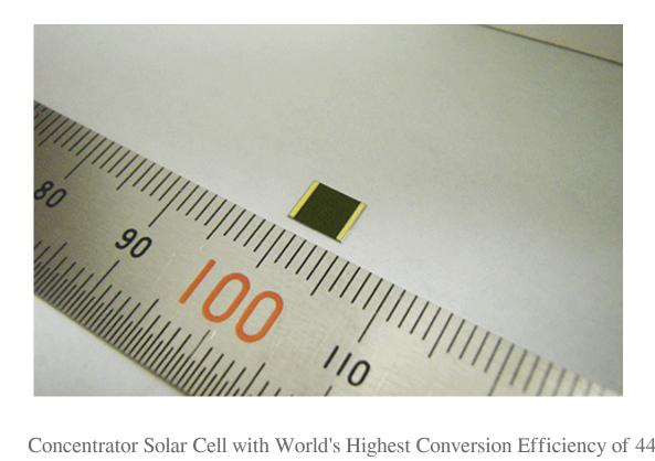
Concentrator Solar Cell with World's Highest Conversion Efficiency of 44.4%.
