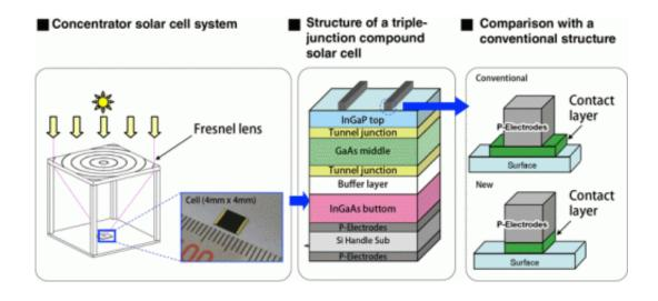
To achieve a concentrating conversion efficiency of 44.4%, Sharp worked to widen the effective concentrator cell surface and ensure uniformity of width at the interface of the connecting concentrator cell and electrodes.
