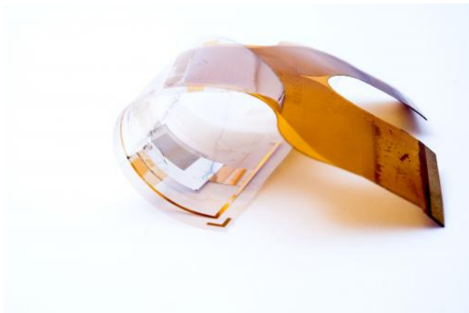
Fully-organic, flexible imager developed by imec, Holst Centre and Philips Research
