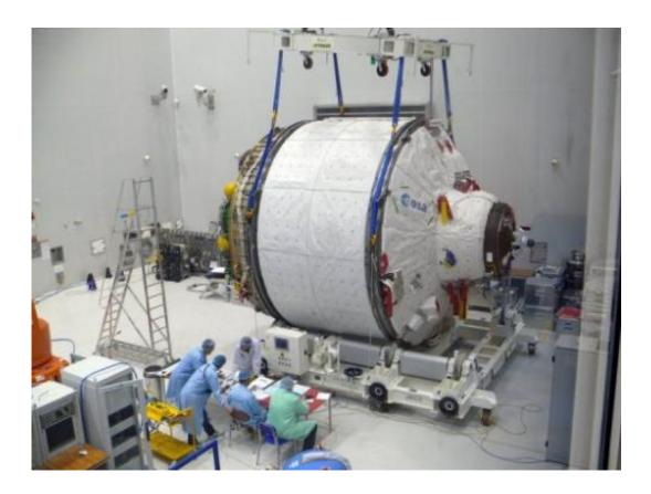
Image provided by the European Space Agency on January 16, 2013 shows the ICC portion of ATV Albert Einstein being weighed at Kourou space center, French Guiana. The main cargo is loaded about five months before liftoff, which requires two days.
