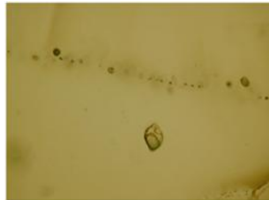
Photo?Under polarizing light microscopy showing fluid inclusions composed of magnesite, saline fluid and vapor bubble in an olivine crystal of the Pinatubo harzburgite. The width is 0.25mm.
