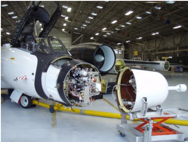
PALMS instrument aboard NASA WB57F. Credit: Karl Froyd, NOAA and CIRES
