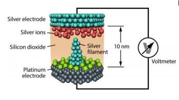
Configuration of a resistive storage cell (ReRAM): An electric voltage is built up between the two electrodes so that the storage cells can be regarded as tiny batteries. Filaments formed by deposits during operation may modify the battery's properties. Credit: Jülich Aachen Research Alliance (JARA)
