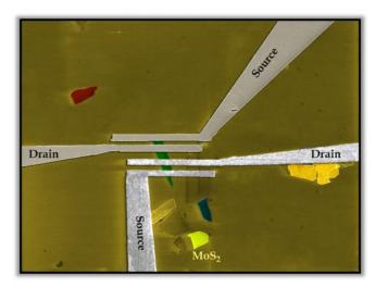
Researchers are developing a new type of semiconductor technology, pictured here, for future computers and electronics based on "two-dimensional nanocrystals." The material is layered in sheets less than a nanometer thick that could replace today's silicon transistors. Credit: Birck Nanotechnology Center, Purdue University
