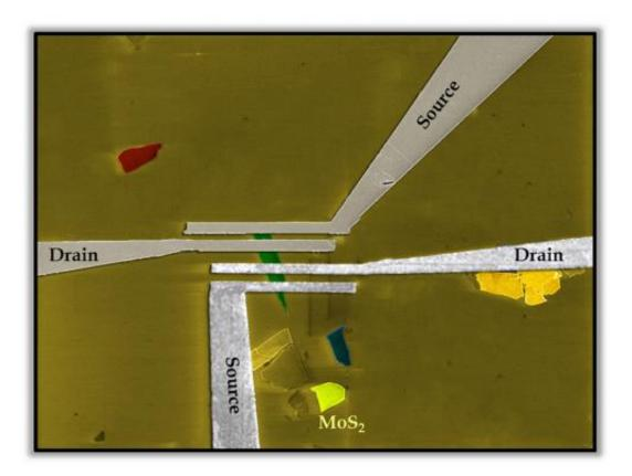
Researchers are developing a new type of semiconductor technology, pictured here, for future computers and electronics based on "two-dimensional nanocrystals." The material is layered in sheets less than a nanometer thick that could replace today's silicon transistors. Credit: Birck Nanotechnology Center, Purdue University
