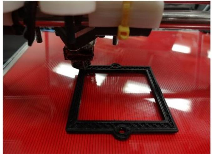
An open-source 3D printer printing an optical component, specifically, a filter bracket.
