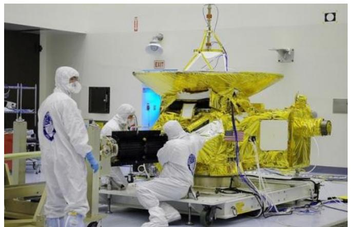
New Horizons in the Payload Hazardous Servicing Facility at the Kennedy Space Center. Note the RTG (black) protruding from the spacecraft. Credit: NASA/Uwe W.
