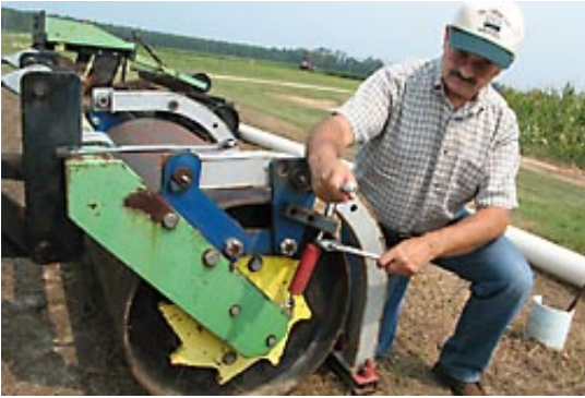
Agricultural engineer Ted Kornecki adjusts the crimping force of his patented smooth roller with oscillating crimping bar. Credit: Ted Kornecki
