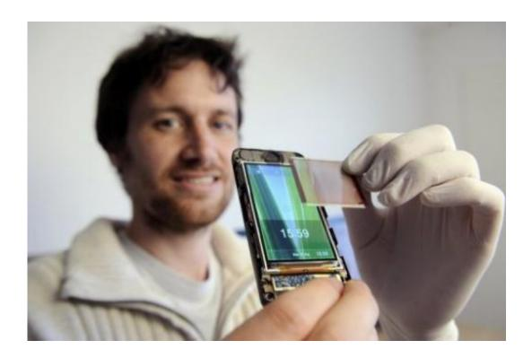
Company head Ludovic Deblois demonstrates Wysips's photovoltaic film in Lambesc, France in 2011. Wysips, a startup based in Aix-en-Provence, southern France, has developed a photovoltaic film which can be built seamlessly into a mobile phone screen and deliver the joy of life to a flat battery.
