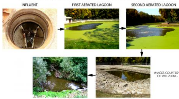
Wastewater, called the influent, is pumped from homes to the sewage treatment facility. This water is then pumped through a series of lagoons, either aerated or not, that contain microorganisms to degrade contaminants like pharmaceuticals, personal care products (PPCPs) and hormones. The water is pumped into a sand tank for further filtration, then the effluent is finally discharged into a creek or other body of water.
