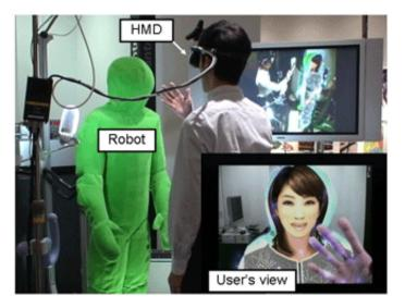
Users see composite images via a head mounted display which has a pair of video cameras inside.
