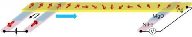
Measuring spin propagation. Two magnetic contacts (left) are used to create a spin polarization (red arrows) at one end of a silver nanowire (yellow), whose value after travelling a defined distance is measured by a third contact. Credit: 2012 Nature Publishing Group
