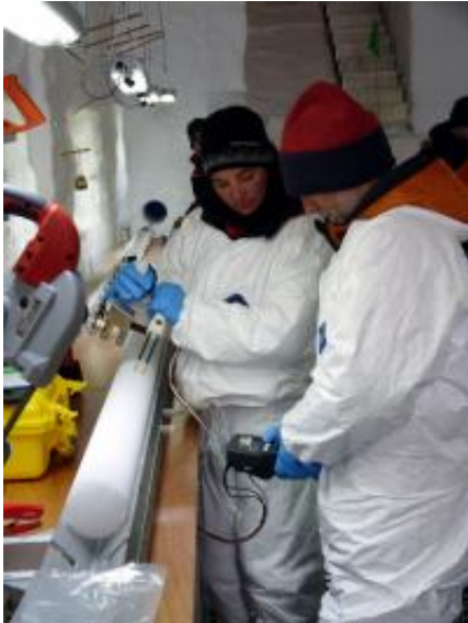
Dr Bertler with German scientist Dr Sepp Kipfstuhl, measuring the electrical conductivity of an ice core.
