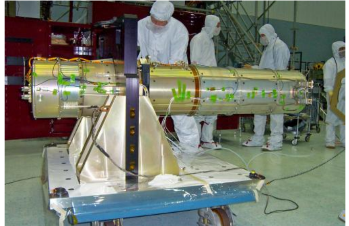
Technicians prepare Swift's UVOT for vibration testing on Aug. 1, 2002, more than two years before launch, in the High Bay Clean Room at NASA's Goddard Space Flight Center in Greenbelt, Md. Credit: NASA's Goddard Space Flight Center
