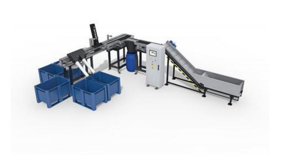
Research at the University of Gothenburg, Sweden and Chalmers University of Technology, Sweden has resulted in a new type of machine that sorts used batteries by means of artificial intelligence. One machine is now being used in the UK, sorting one-third of the country?s recycled batteries. Credit: Claes Strannegård
