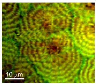
Typical BCARS composite image of a polyethylene blend taken at NIST showing circular polarization response. LLD polyethylene shows red in this mode, while the HD polyethylene with deuterium substituted for hydrogen is green. Credit: NIST
