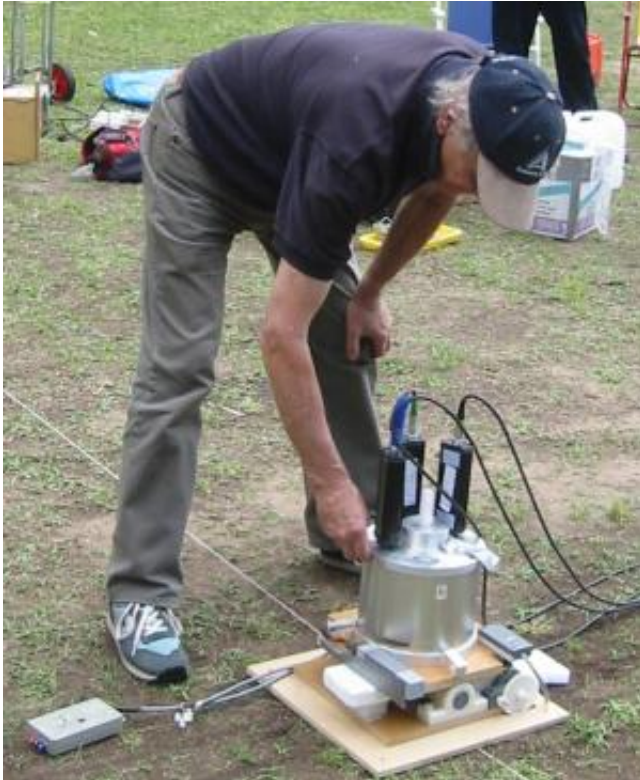
CSIRO researcher, Keith Leslie, prepares the magnetic sensor for field trials.
